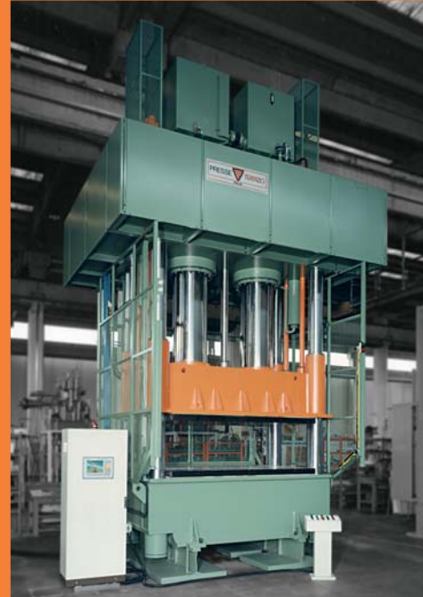
Column press KOMPO 1200 SMC Platens 2600x1850
