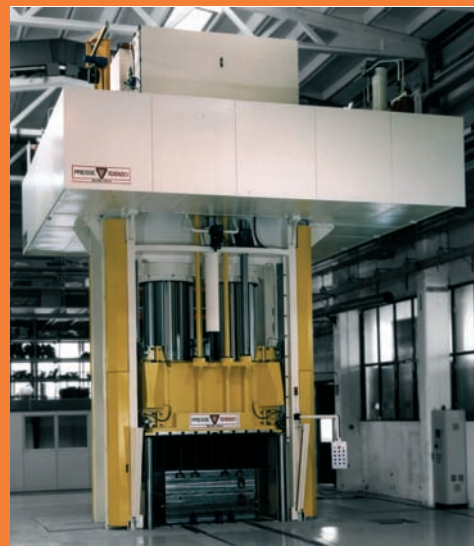
KOMPO 3000 GMT Platens 2700x2000 with control of parallelism
