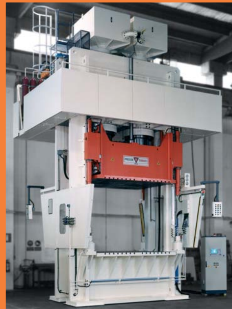
Frame press KOMPO 2000 SMC Platens 3000x2500 with control of parallelism
