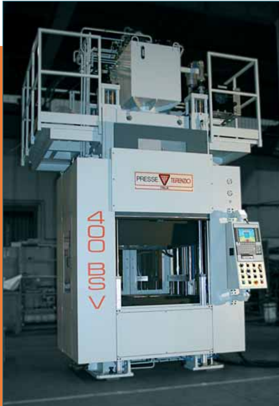
Press 400BS.V platens 800x800 with vacuum chamber and ejection side bars.
